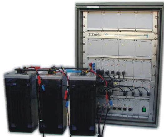
Fig. 1. The multi-channel impedance spectroscopy EIS meter (shown with industrial lead–acid batteries) is used to carry out impedance measurements on batteries, supercapacitors and fuel cells with up to 14 simultaneous impedance measurements on half-cells, cells, stacks or blocks.
